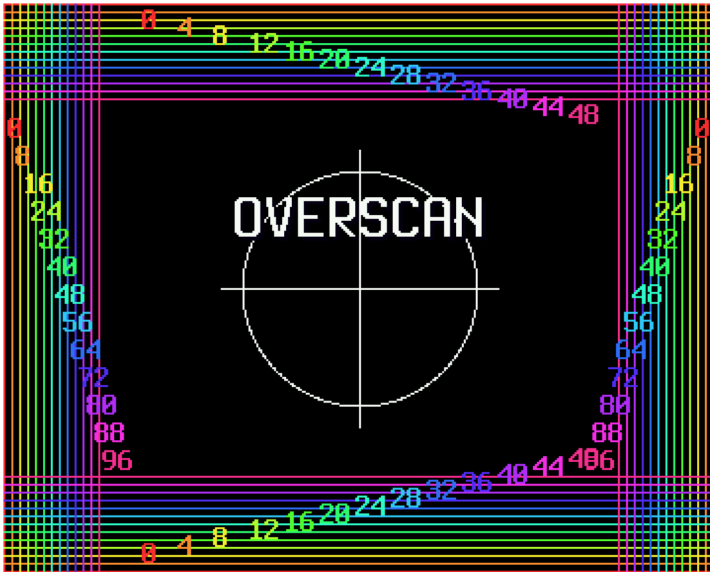
Figure 2: The test card: numbered lines on every edge, read off the tube by a human.
